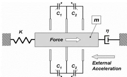
Figure 5. Schematic mechanical system of a capacitive accelerometer
